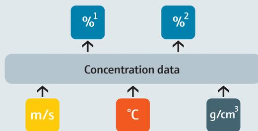
The concentration of both, the cleaner and the bath contamination, can be determined in-line with the right concentration data by combining the temperature, speed of sound and acoustic density. Concentration data are created to customer specification in our applications laboratory. We make use of intelligent evaluation algorithms based on multivariate data analysis.
