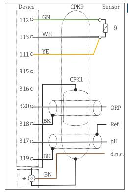
€ 40 Wiring diagram For rH measurement, connect a pH sensor (e.g. CPS11 with CPK9 sensor cable) and an ORP sensor (e.g. CPS12 with CPK1 sensor cable).
