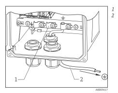
Cable mounting rail ≥2.5 mm² (14 AWG) functional ground
