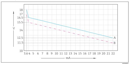
$\blacksquare$  9 Minimum supply voltage at the transmitter depending on the output current
