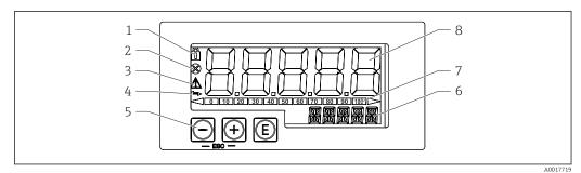
■ 14 Display and operating elements of the process display unit
