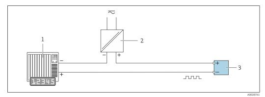
■ 12 Connection example for pulse/frequency output (passive)
