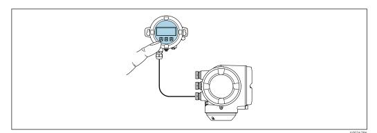
lacktriangle 35 Operation via remote display and operating module DKX001
