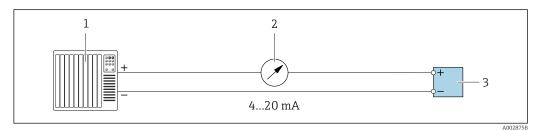
■ 10 Connection example for 4-20 mA current output (active)
