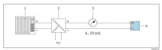
■ 11 Connection example for 4-20 mA current output (passive)
