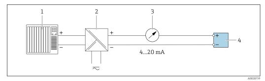
■ 11 Connection example for 4-20 mA current output (passive)
