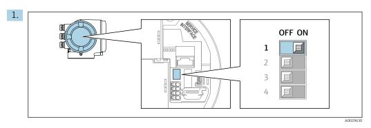
Setting the write protection (WP) switch on the main electronics module to the **ON** position enables hardware write protection.
