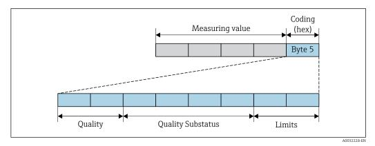
■ 35 Structure of the coding byte
