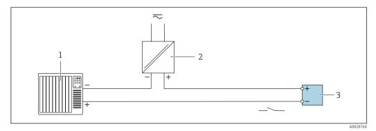
■ 20 Connection example for relay output (passive)
