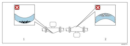
■ 7 Orientation of sensor with curved measuring tube
