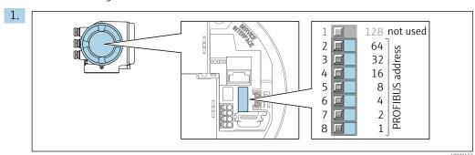
Set the desired device address using the DIP switches in the connection compartment.
