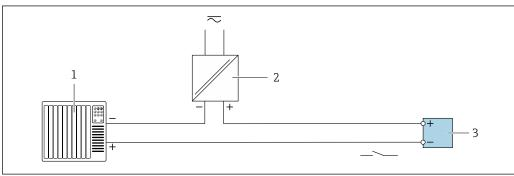
2 19 Connection example for switch output (passive)
