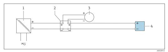
■ 21 Connection example for 4 to 20 mA current input
