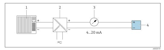
■ 17 Connection example for 4-20 mA current output (passive)
