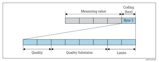
■ 29 Structure of the coding byte
