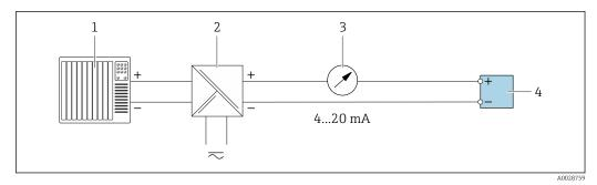
■ 12 Connection example for 4-20 mA current output (passive)
