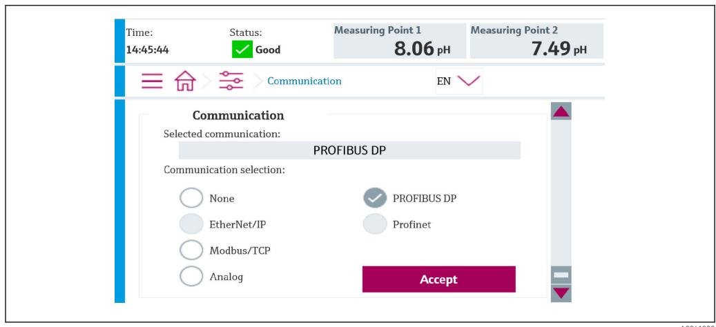
**i** Only one fieldbus communication is used to send commands to the Liquiline Control CDC90 or to read the values.
