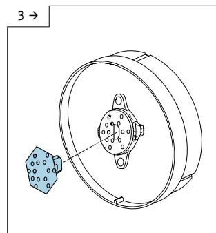
► **For Promass:** Insert S-DAT into the ISEM electronics module.
