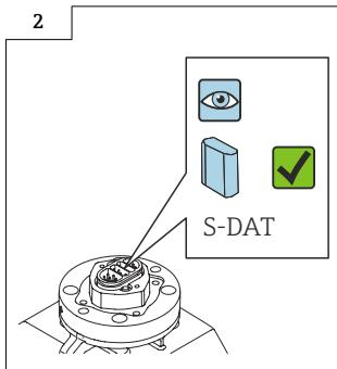
**i** Otherwise, remove the S-DAT from the defective amplifier (Fig. 1 below) and install it in the new amplifier (Fig. 2 or 3 below).
