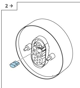
► **For Promag:** Insert S-DAT into the ISEM electronics module.
