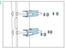
Fit the counterparts and fasten the post retainer using spring washers and nuts.
