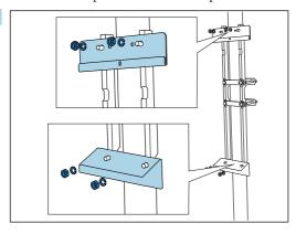
Mount the wall holder unit (included in the delivery with the analyzer) on the post retainer.
