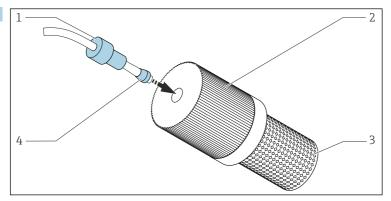
■ 20 Mounting the suction strainer (supplied) on the sample hose
