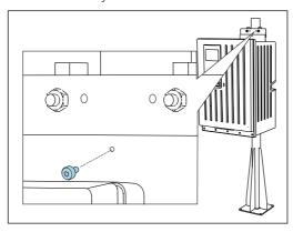
Fix the upper wall holder unit in place with the screw provided.
