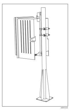
■ 12 Analyzer mounted on post (from front)
