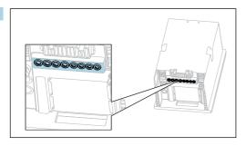
Guide the cables through the cable glands on the bottom of the device.
