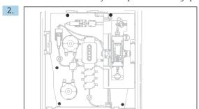
Release the 5 screws on the carrier board using a Torx screwdriver (T25).
