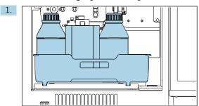
Remove the bottle tray: Lift up the recessed grip slightly and pull it towards the front.
