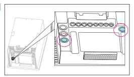
Guide the heated waste hose (left in the graphic) and the heated sample hose (right in the graphic) through the cable glands indicated.
