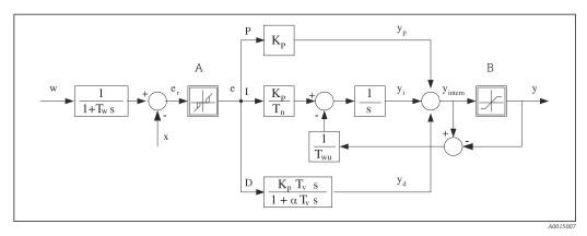
75 Block diagram of the controller structure
