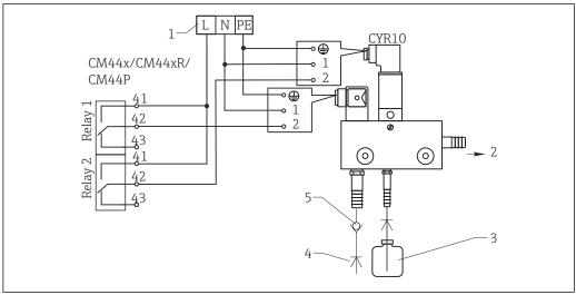
€ 48 Connecting the CYR10 injector cleaning unit
