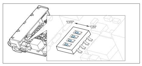
■ 51 DIP switch for internal termination
