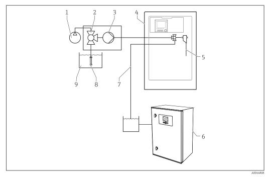
$\blacksquare$  8 Measuring system with Liquiline System CA80, Liquiline System CAT820 and second analyzer
