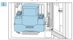
Remove the bottle tray: Lift up the recessed grip slightly and pull it towards the front.
