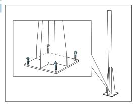
Erect the post and mount it securely on the foundation using 4 fixing screws (to be provided by the customer  $^{1}$ ).
