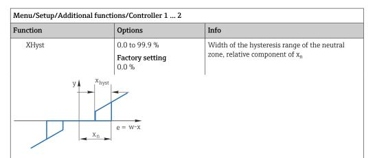
The graphic illustrates the manipulated variable (with a pure P-controller) over the control deviation e (set point minus controlled variable). Very low control deviations are set to zero. Control deviations  $> x_n$  are processed "in the normal way". Via  $x_{hyst}$  it is possible to configure a hysteresis to suppress oscillations at the edges.
