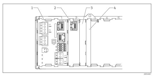
**■** 32 Connection compartment in the controller housing
