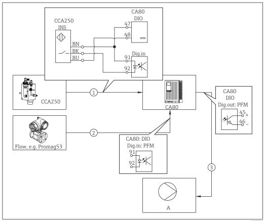
■ 65 Example of chlorine control with feedforward control
