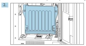
Remove the cover that is hooked into place.
