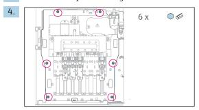
Release the 6 screws of the carrier board using an Allen key.
