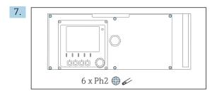
Release the 6 screws on the electronics compartment cover using a Phillips-head screwdriver and fold out the cover towards the front.
