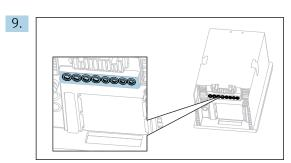
Guide the cables through the cable glands on the bottom of the device.
