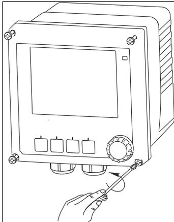
Loosen the 4 screws on the front with a Phillips head screwdriver.
