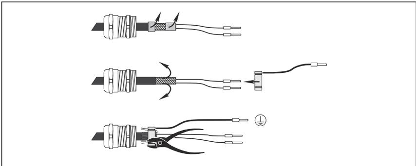
2. Connect the stranded extension wire to the cable mounting rail.
