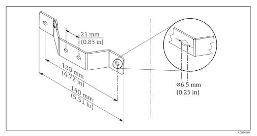
Dimensions of angle bracket for wall mount (complete wall mounting set available as accessory)
