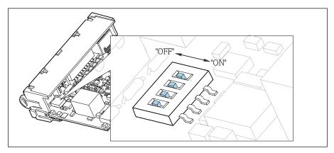
■ 51 DIP switch for internal termination
