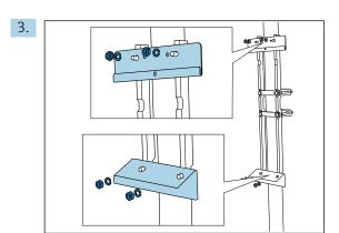
Mount the wall holder unit (included in the delivery with the analyzer) on the post retainer.
