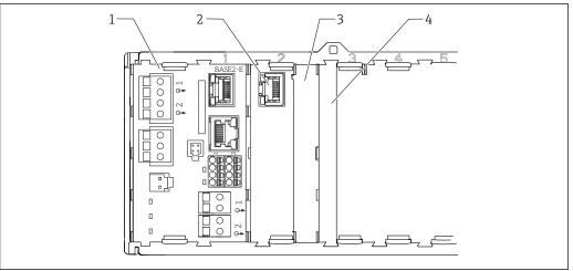
**■** 32 Connection compartment in the controller housing
