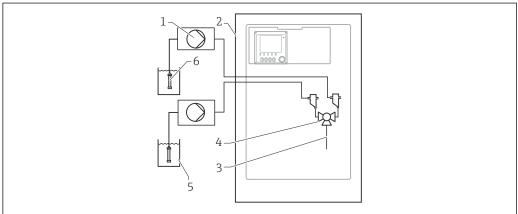
Measuring system with 2x Liquiline System CAT820
