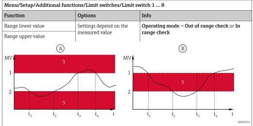
ightharpoonup 70 Range monitoring outside (A) and within (B) a range (without hysteresis and switch-on delay)
