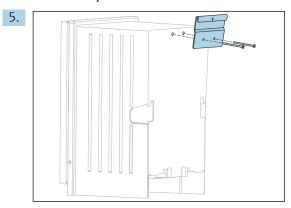
Screw the suspension bracket of the wall holder unit (included in the delivery with the analyzer) onto the analyzer.
