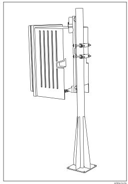
■ 23 Analyzer mounted on post (from front)
