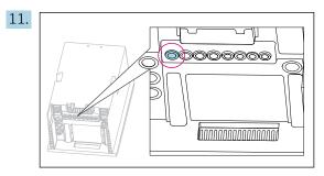
Guide the power supply cable, which is provided by the customer at the installation location, through the cable gland indicated.
