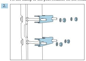
Fit the counterparts and fasten the post retainer using spring washers and nuts.
