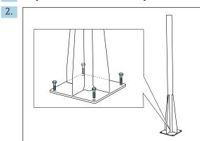
Erect the post and mount it securely on the foundation using 4 fixing screws (to be provided by the customer  $^{1}$ ).
