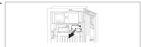
7. Connect the cleaning valve to the following plug-in terminals:
