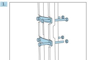
Fit the clamp of the post retainer on the retaining rods and post using the nuts.
