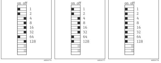
🛮 53 Valid PROFIBUS address 67 📵 54 Valid Modbus address 195 📵 55 Invalid address 255 🗓
