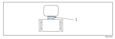
Position of reference point for temperature measurement
