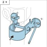
► Mark the distance between the holes on the wall before drilling.
