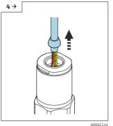
▶ Pull out the cable with the cone.
