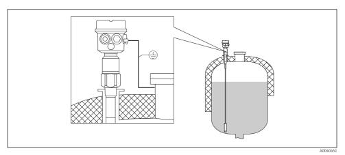
■ 2 A probe with inactive length for the insulated tanks
