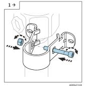
► Screw together the wall bracket on the tube.
