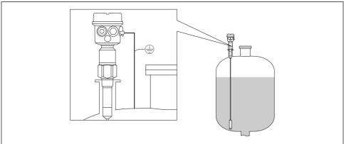
■ 3 A probe with fully insulated inactive length for mounting nozzles
