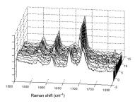
Figure 3: Waterfall plot of Raman spectra. (Copyright © 2004 John Wiley & Sons and the American Pharmaceu-tical Association. Reprinted from Ref. 4 with permission from Wiley-Liss, Inc., a subsidiary of John Wiley & Sons, Inc.)
