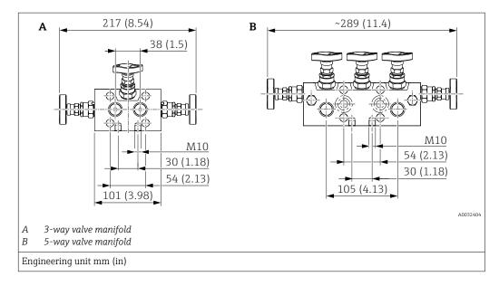
3-way or 5-way valve manifolds in 316L or AlloyC can be ordered
