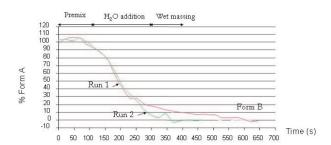
Figure 2: Predicted form conversion, form A to B. In Run 1, the chopper was turned on after water addition. In Run 2, the chopper was on during and after water addition. (Reprinted with permission from Ref. 1. © 2006 Russell Publishing.)
