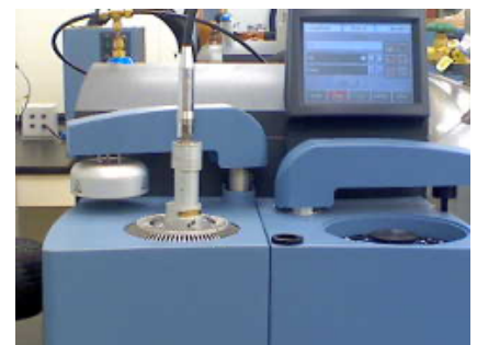
Figure 1: DSC-optimized Raman probe interfaced to the Q2000 DSC
