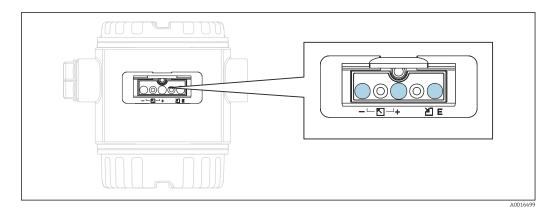
The operating keys on the outside of the device make it unnecessary to open the housing. This guarantees:
