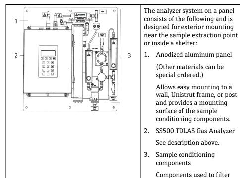
SS500 TDLAS Gas Analyzer with SCS on a panel
