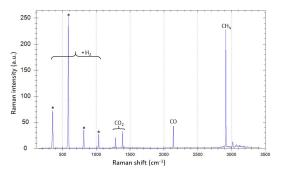
Figure 2: Typical Raman spectrum for syngas
