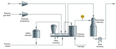
Figure 1: Primary steam reformer section of HyCO plant process units\*\*
