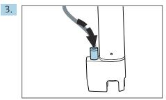
Connect the hose for the compressed air supply (to be provided onsite) or compressor ( $\Rightarrow \implies 30$ ) to the hose connection of the cleaning unit.
