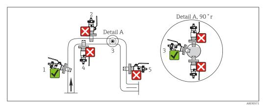
11 Permissible and impermissible sensor installation positions with retractable assembly COA451
