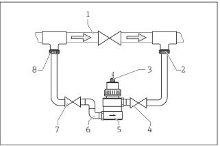
Bypass installation with manually actuated valves or solenoid valves
