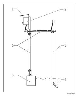
**₽** 6 Assembly holder with immersion tube
