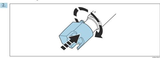
Screw on the cleaning unit or optional protection guard and tighten until the stop.
