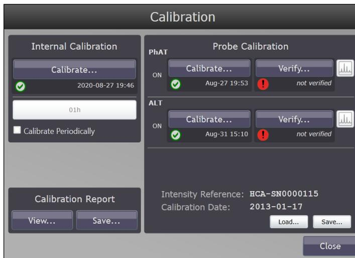
Figure 23. Calibration window with quick view buttons for a Raman Rxn Hybrid analyzer
