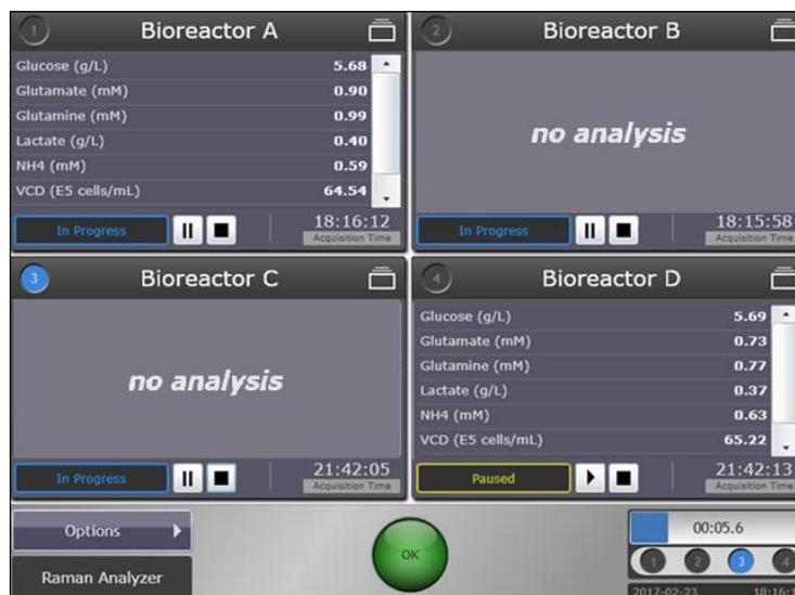
Figure 66. Results for an Rxn4 four channel analyzer with models active for probe 1 and probe 4
