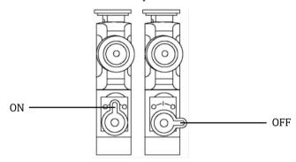
Figure 1. Rxn-10 probe showing the ON and OFF shutter positions
