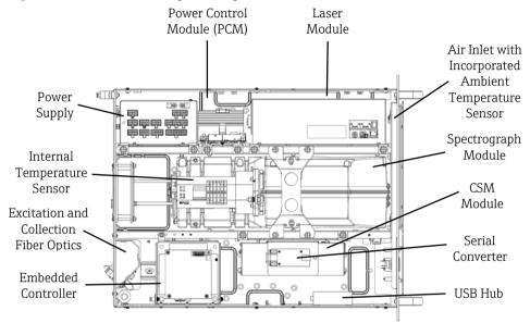
Figure 8. The interior of the Raman Rxn4 analyzer
