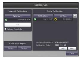
Figure 15. Calibration window with quick view buttons for a Raman Rxn single channel analyzer
