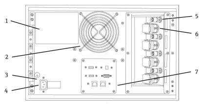
Figure 6. Rear panel of Raman Rxn4
