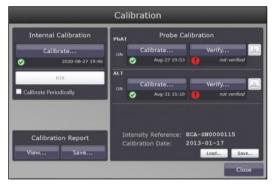
Figure 16. Calibration window with quick view buttons for a Raman Rxn Hybrid analyzer
