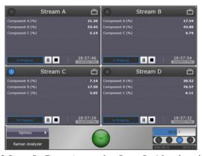
Figure 13. Raman RunTime main screen for a Raman Rxn4 four channel analyzer
