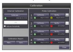
Figure 14. Calibration window with quick view buttons for a Raman Rxn four channel analyzer
