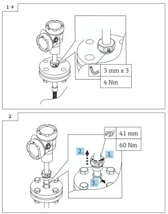
► Be sure to place the C-ring at the bottom of the flange.
