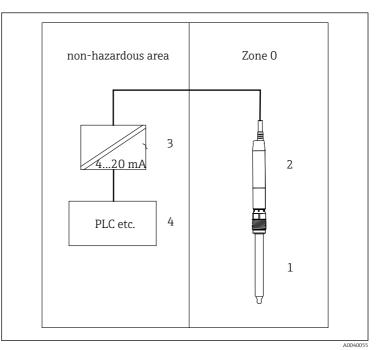
■ 1 Installation in hazardous area: CM82/CM72 and sensor in explosive gas atmosphere
