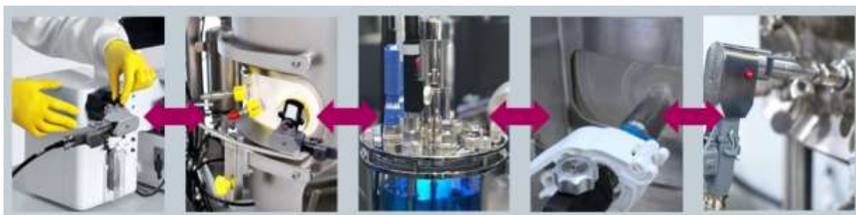
Figure 3: Example of cross-scale Raman analysis using analyzers and bioprocessing probes designed to facilitate scalability from micro and mini bioreactor systems through to single-use and traditional bioreactors of all sizes
