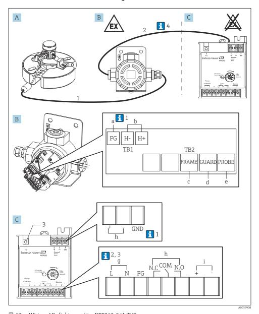
■ 17 Wiring of Ex [ia] transmitter NRR262-2/A/B/C
