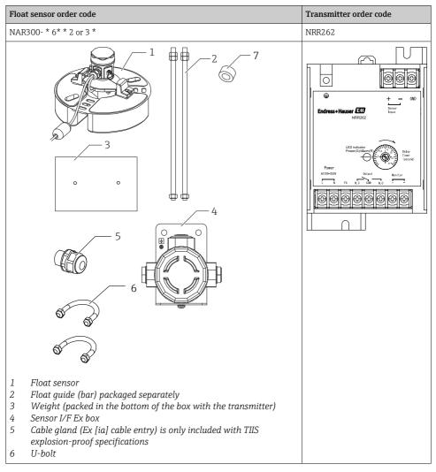
The sensor I/F Ex box is included in the order code NAR300-x6xxxx. The intrinsically safe system is used in combination with NRR262.
