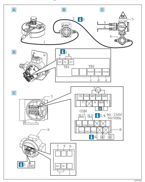
■ 18 Wiring of Ex d [ia] transmitter NRR261-3
