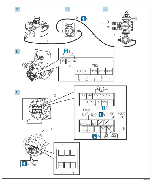
☑ 9 Wiring of Ex d [ia] transmitter NRR261-3
