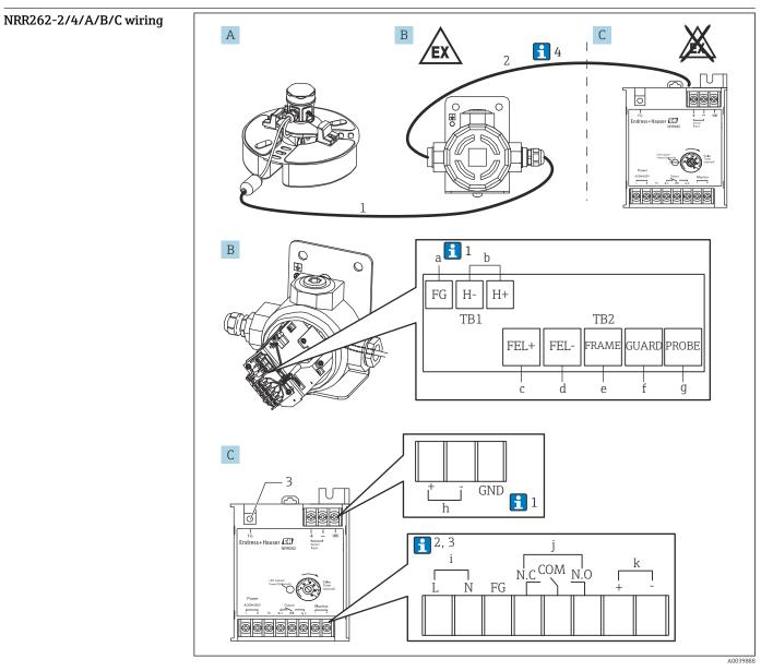
■ 8 Wiring of Ex [ia] transmitter NRR262-2/A/B/C
