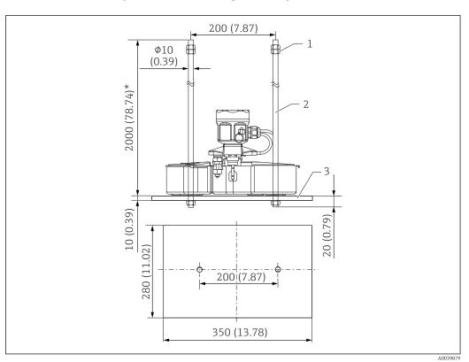
■ 21 Float guide. Unit of measurement mm (in)
