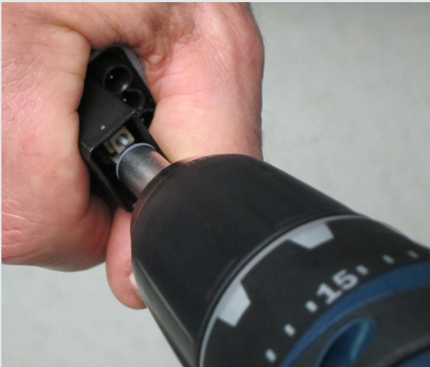
Polishing a fiber in its Harting connector
