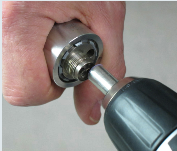
Polishing a fiber inside a Rxn-30 probe
