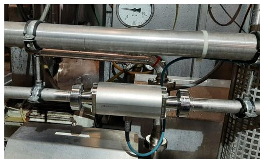
Teqwave H monitors sugar concentration directly in the filling process
