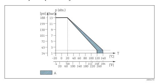
**■** 4 *Mechanical pressure-temperature resistance*
