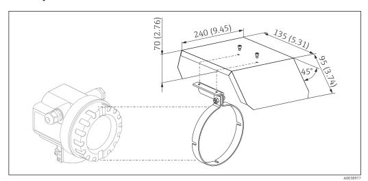
$\blacksquare$  36 Weather protection cover for F12 or T12 housing . Unit of measurement mm (in)
