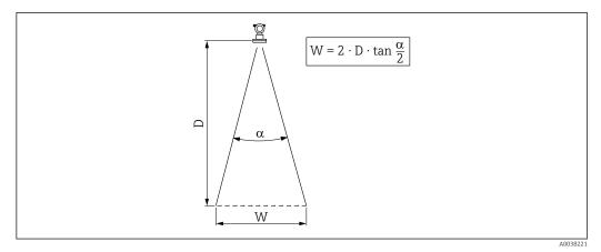
$\blacksquare$  8 Relationship between beam angle  $\alpha$ , distance D and beamwidth diameter W
