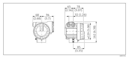
■ 18 Dimensions of T12 housing. Unit of measurement mm (in)
