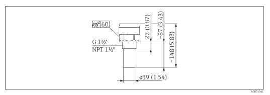
Dimensions of FMU40 sensor. Unit of measurement mm (in)
