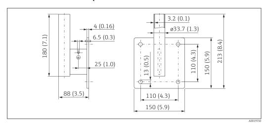
$\blacksquare$  31 Dimensions of the wall bracket. Unit of measurement mm (in)
