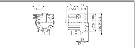
$\blacksquare$  17 Dimensions of F12 housing. Unit of measurement mm (in)
