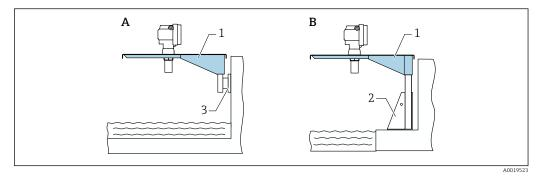
■ 34 Cantilever with mounting stand or wall bracket
