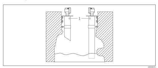
$\blacksquare$  9 Installation in narrow shafts with very uneven shaft walls
