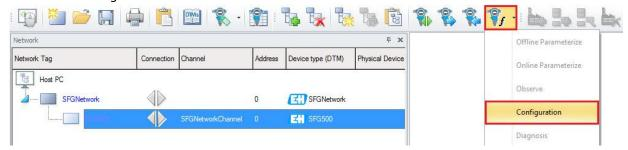
• Configure the IP address of the SFG500 as well as the scanning range. In this example, the SFG500 IP address is 10.126.104.253 and the scanning range is set between PROFIBUS address 10 and 46:
