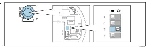
Switch DIP switch no. 3 to **On**.
