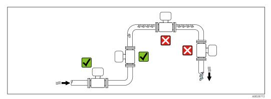
To prevent measuring errors arising from accumulation of gas bubbles in the measuring pipe, avoid the following mounting locations in the piping:
