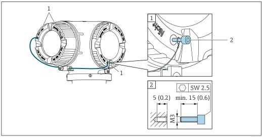
Cover borehole for the securing screw
