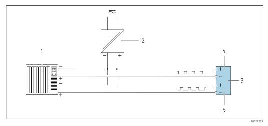
■ 16 Connection example for double pulse output (passive)
