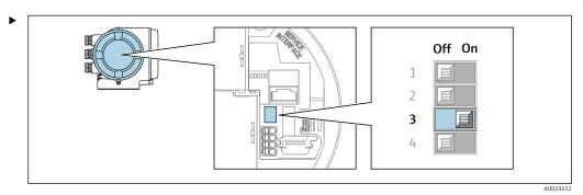
Switch DIP switch no. 3 to **On**.
