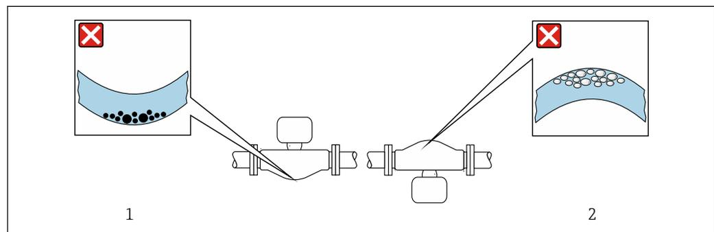
☒ 23 Orientation of sensor with curved measuring tube
