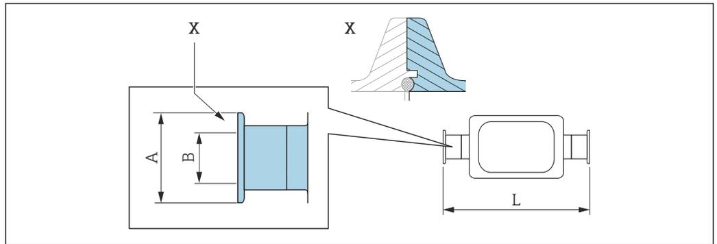
45 Detail X: Asymmetrical process connection; the part shown in blue is provided by the supplier.
