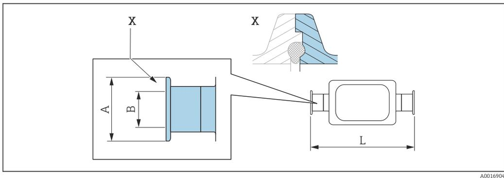
44 Detail X: Asymmetrical process connection; the part shown in blue is provided by the supplier.
