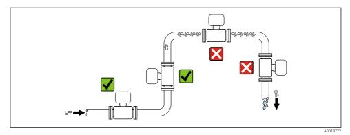
Installation in down pipes
