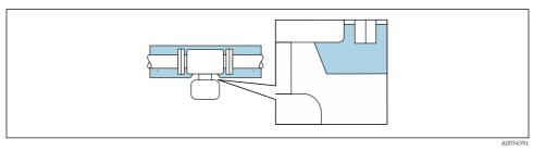
3 Thermal insulation with not isolated extended neck
