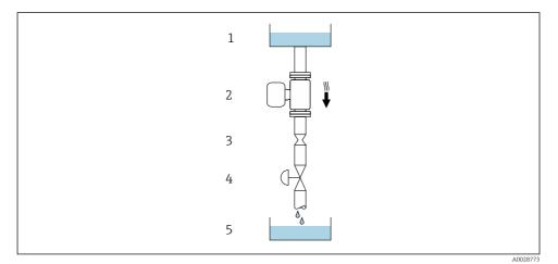
2 Installation in a down pipe (e.g. for batching applications)
