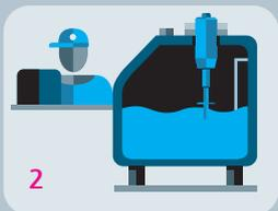
**Calibration** Qualified staff have to disassemble the sensor and calibrate it in a mobile block calibrator with a traceable reference (master).
