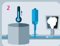
**Reference measurement** The master utilizes the Curie temperature principle. Falling short of this value – such as after cleaning with steam – initiates calibration.
