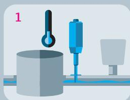
**Self-monitoring** A special reference sensor – the master – allows for a one-point calibration of the primary temperature sensor in the ongoing process.
