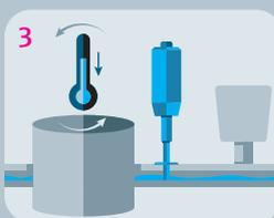
**Operation** The process is not interrupted; the system is not opened up. Staff need only intervene if iTHERM TrustSens reports a malfunction.
