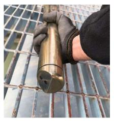
Turbimax CUS52D turbidity sensor installed in recovered water open channel, assembly installation is carried out in mechanical structure of the bridge of the thickener N°2
