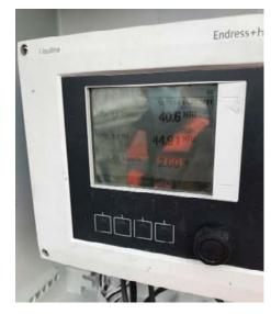
Liquiline CM442 showing measured values: Channel 1: Turbimax CUS50D (Tested device) measured values are below the measuring range of the device. Channel 2: Turbimax CUS52D. Channel 3: Turbimax CUS71D
