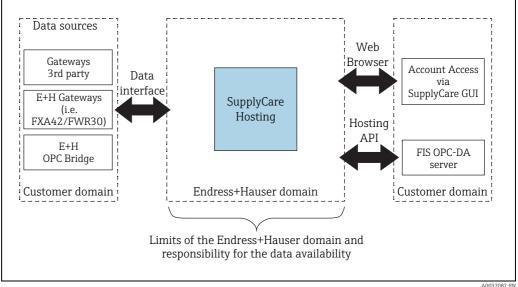
To connect to the Endress+Hauser hosting system, customers use the Internet. The responsibility transfer point for data communication between the customer's IT infrastructure and the hosting system operated by Endress+Hauser is described in the diagram above.
