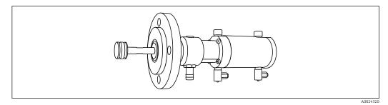
■ 11 Samplefit CSA420 sampling assembly with flange connection DN50, PP
