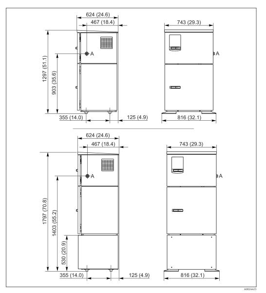
26 Dimensions of Liquistation, stainless steel version, without/with stand. Unit of measurement mm (in)
