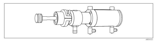
■ 12 Samplefit CSA420 sampling assembly with Triclamp connection DN50, DIN 32676
