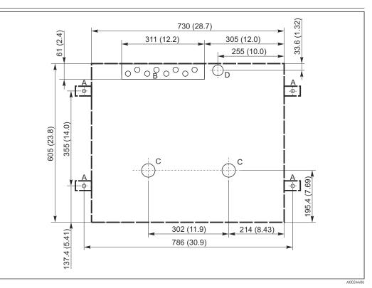
፼ 22 Foundation plan. Unit of measurement mm (in)
