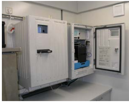
Compact installation of orthophosphate and total phosphorous analyzer CA80PH / CA80TP in the container (top)
