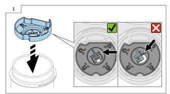
Connect the connecting cable to the sensor. Slide the plastic insulation over the connecting cable. Carefully turn the housing until the profile is positioned in the groove. Then continue to turn the housing carefully until the end stop of the sensor assembly.
