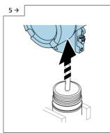
Carefully remove the housing from the sensor assembly, taking care not to damage the sensor cable.
