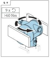
Unscrew the housing using a high degree of force (> 60 Nm). This involves applying force several times in and against the screw direction; the snap ring is intentionally destroyed in the process.
