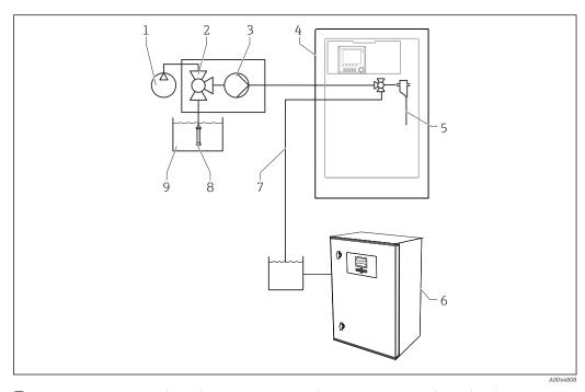
₽8 Measuring system with Liquiline System CA80, Liquiline System CAT820 and second analyzer
