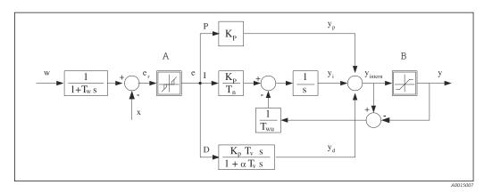
■ 77 Block diagram of the controller structure
