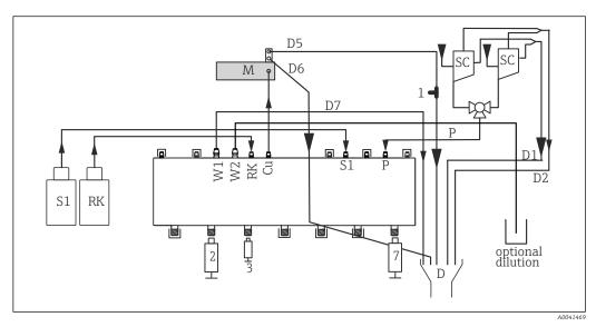
■ 65 Liquiline System CA80PH (molybdate-vanadate method), two-channel device
