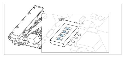
■ 53 DIP switch for internal termination
