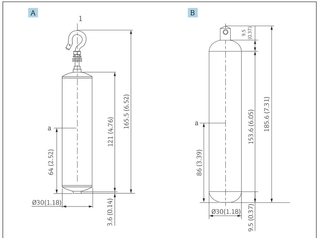
A Displacer cylindrique Ø30 mm (1,18 in), 316L
