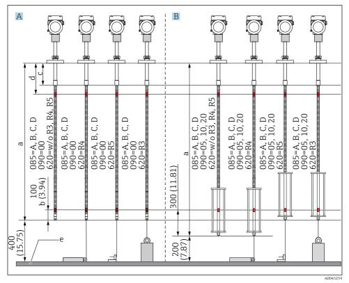
Position of NMT81 element No. 1 based on the installation method. Unit of measurement mm (in)
