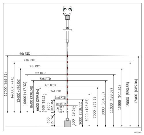
■ 11 Elemement position. Unit of measurement mm (in)
