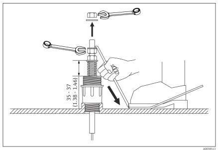
■ 24 Top anchor installation 2. Unit of measurement mm (in)
