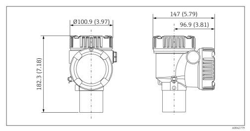
**■** 3 Standard converter. Unit of measurement mm (in)
