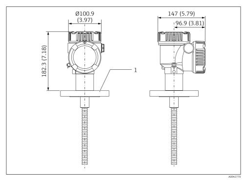
■ 8 Welded flange. Unit of measurement mm (in)
